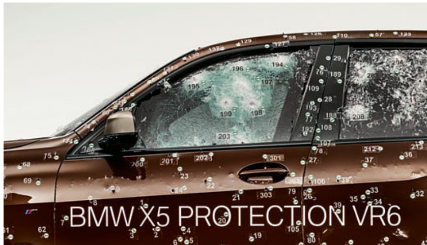
Multi-layer safety glass: The driver and passengers of the new BMW X5 Protection VR6 are protected by an approximately 30 mm thick multi-layer safety glass with an internal polycarbonate splinter protection layer.
