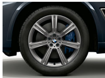
■ 20" light alloy wheels Star-spoke style 736 Ferric Grey with mixed tyres and runflat tyres, front 9J x 20 with 275/45 R20 tyres, rear 10.5J x 20 with 305/40 R20 tyres.
